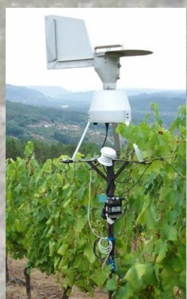
Figure 4. Aerobiological sensor station at the vineyard level.
